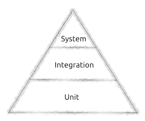
This diagram has probably been drawn thousands of times. Although unit tests will appear at the bottom of each version, the words used at the other levels will vary wildly.
